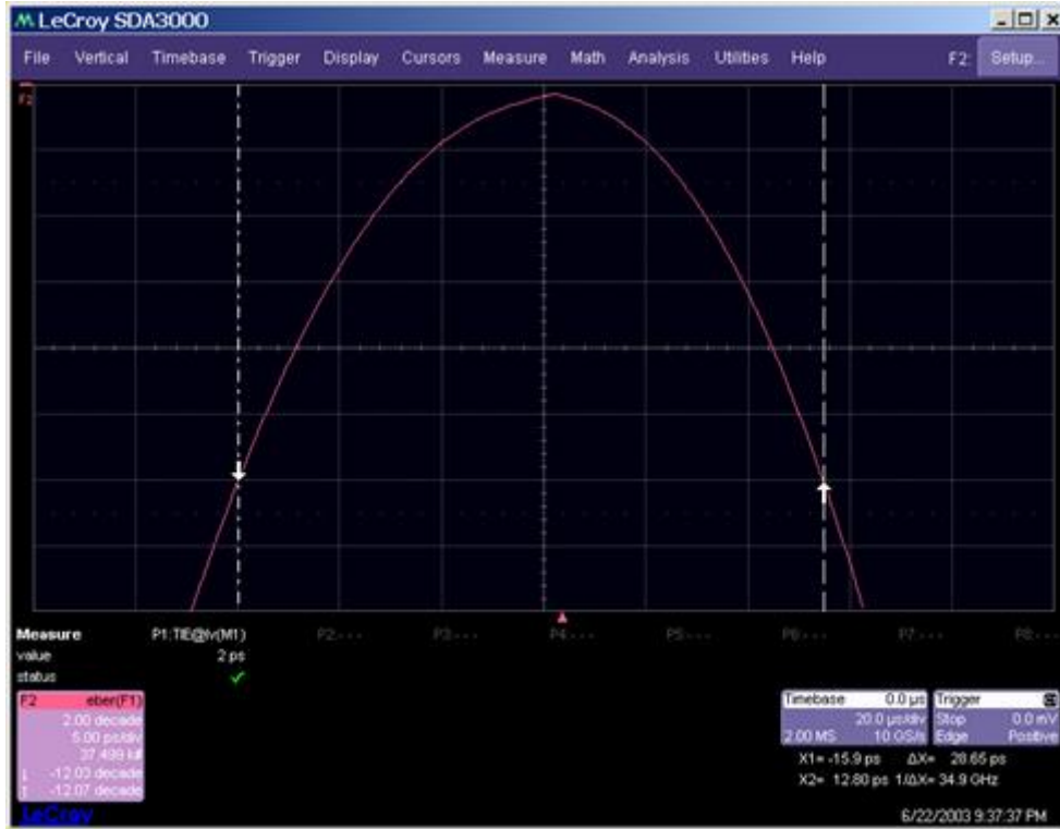
Figure 9. Total jitter curve. The vertical values of this curve represent the probability of a data transition occurring at a time represented by the horizontal axis. The horizontal center of the plot is 0 ps. The two markers are placed at the vertical level corresponding to a bit error rate of 10 \text{ e-}12 and the horizontal distance between these two points is the total jitter at this bit error rate.
